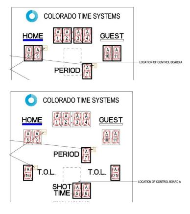
2. Set the Channel and PAN on the dip switches for control board A.
