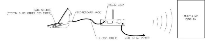
When using a wireless connection, the WA-2 wireless adapter and scoreboard must be set to the same channel and PAN. Follow the WA-2 user instructions to change its channel and PAN. Follow instructions on previous pages if scoreboard Channel and PAN must be changed.
